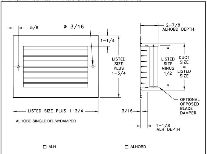
This series of horizontal adjustable face bar grilles and registers are made of extruded aluminum. Available with or without opposed blade damper. White (WHT) or clear anodized (CLR) finishes are available. Z-Frame is available as a special order.
