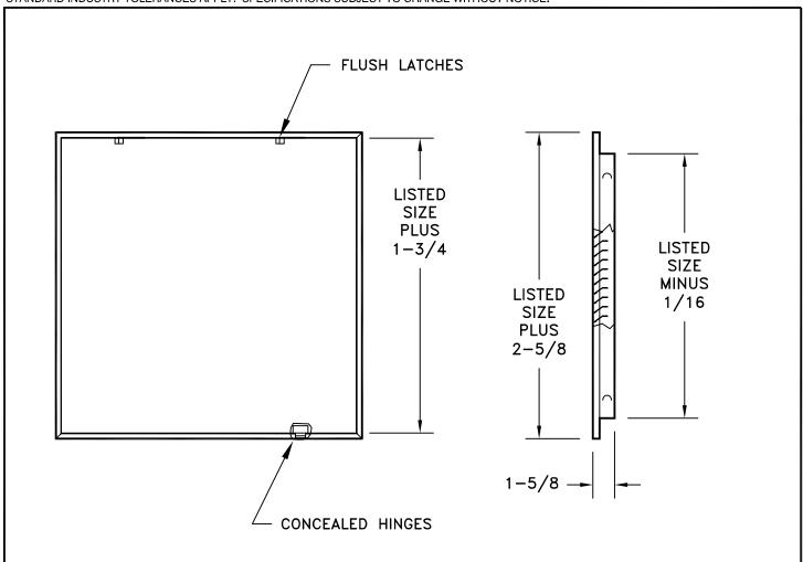
Model LAD has a removable stamped face with concealed latches and hinges. Finish: White (W) Available Sizes-6X6,8X8,10X10,12X12,14X14,16X16,24X24 Face is 22 Gauge. The Frame is 24 Gauge
